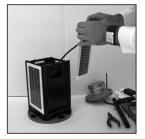
9. Recommended torque settings for Fitment of Light Heads to Solar Base units using the 4 Hex Bolts supplied. It is recommended that the bolts for holding the light heads to the Solar Base units have a torque setting applied of 3Nm for a satisfactory seal.
